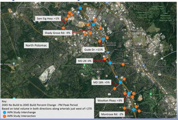
This graphic shows the changes in two-directional traffic volume just west of I-270 along the roadways that have interchanges with I-270 along the Phase 1 South limits.
